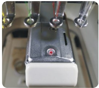
◎ 红光定位装置 Red laser positioning device
