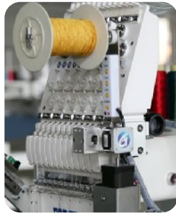
◎ 简易绳绣 Easy cording device
