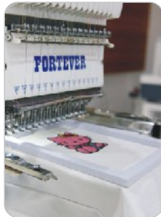
◎ 八合一磁铁绣框 8 in 1 magnetic frame
