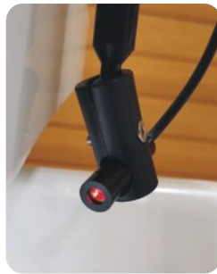
◎ 红光定位装置 Red laser positioning device
